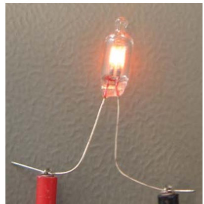
Figure 2 Neon lamps served as references before IC-semiconductor engineers designed solid-state voltage regulators in the 1960s (courtesy www.giangrandi.ch).
