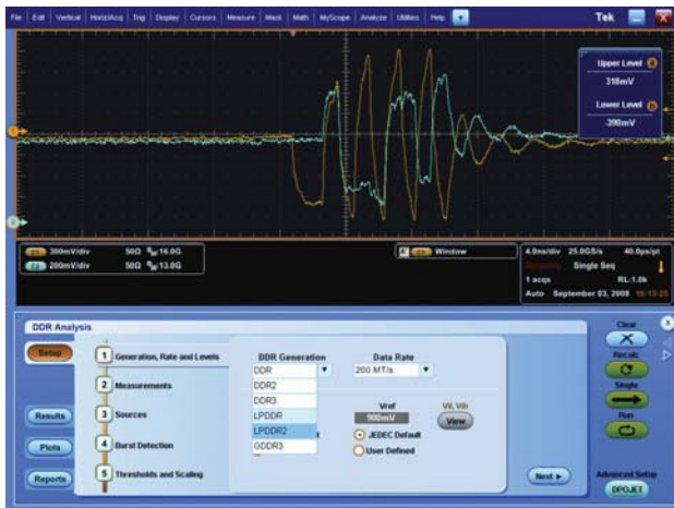
Figure 5 To ease setup tasks, a menu-driven interface guides you through a selection process.
