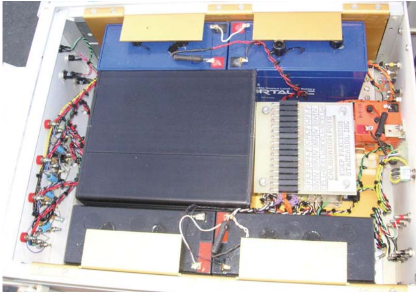
Figure 10 This four-cell voltage reference, which the late Kenneth Koep designed, uses batteries to keep the circuit operating when unplugged. The zener reference cells are in constant-temperature ovens, and you can average the four cells to reduce noise and improve accuracy.
